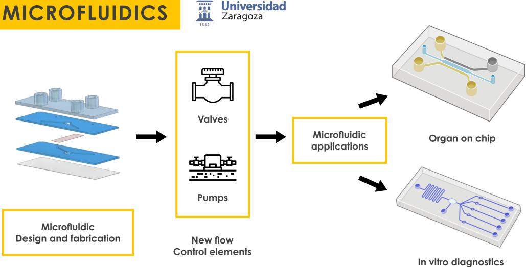
PRIME will implement integrated valves and pumps with active fluidic elements that allow an accurate flow control for microfluidic applications
