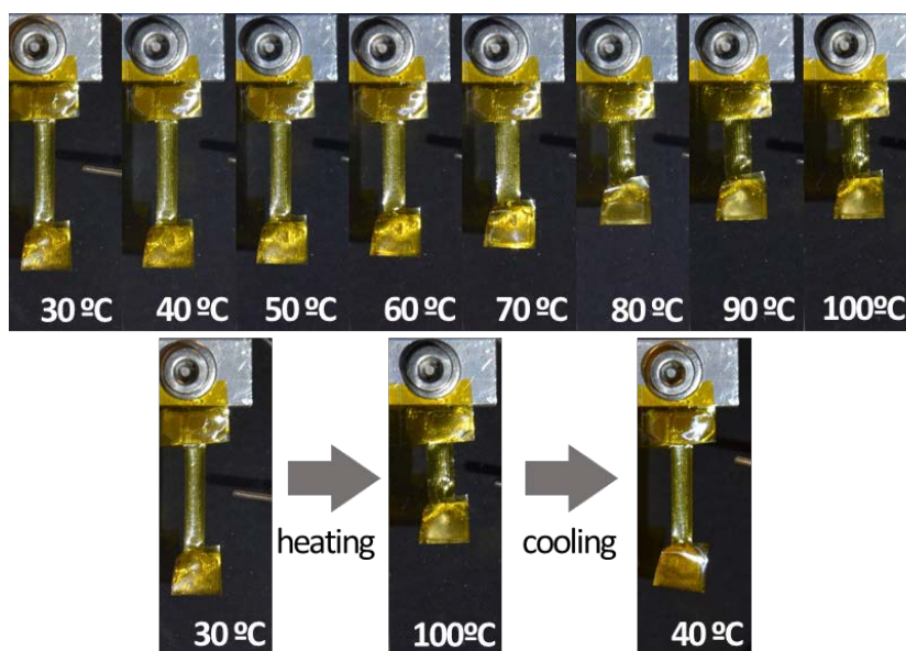
Figure 14, Top: Thermomechanical deformation of a free-standing sample. Sample printed having a shape of a dog bone. Bottom: Sample after heating to 100 °C and its relaxation through cooling down to 30 °C.
