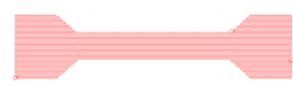
Figure 9, Schematic representation of LCE samples. The dog-bone model is consisting of continuous stripes of ink with uniaxial orientation. It contains closely packed parallel lines (150 \mu\text{m} ) along one direction (long side).
